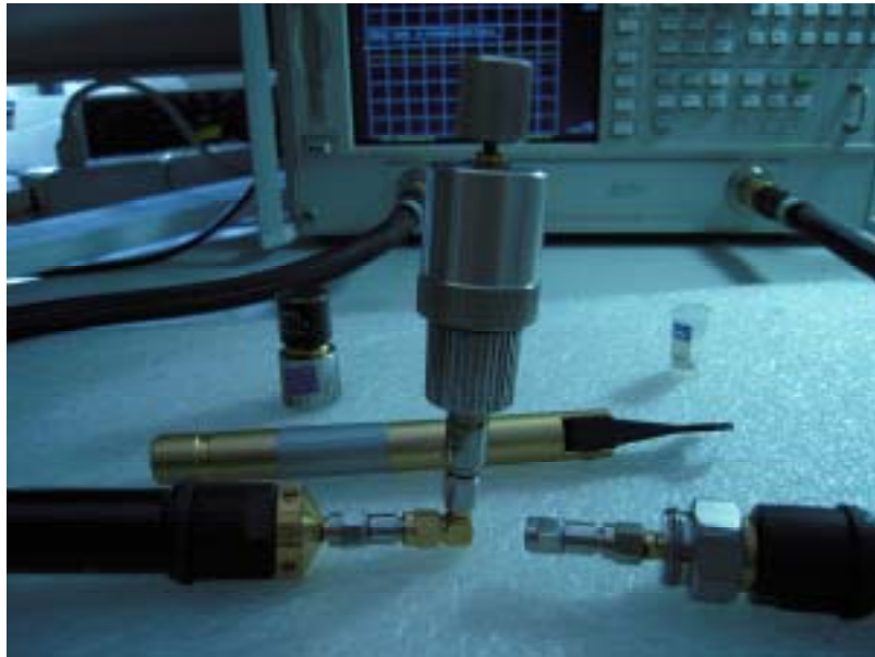
Figure 2. 17 The special designed test fixture for the measurement of the chip capacitors.
