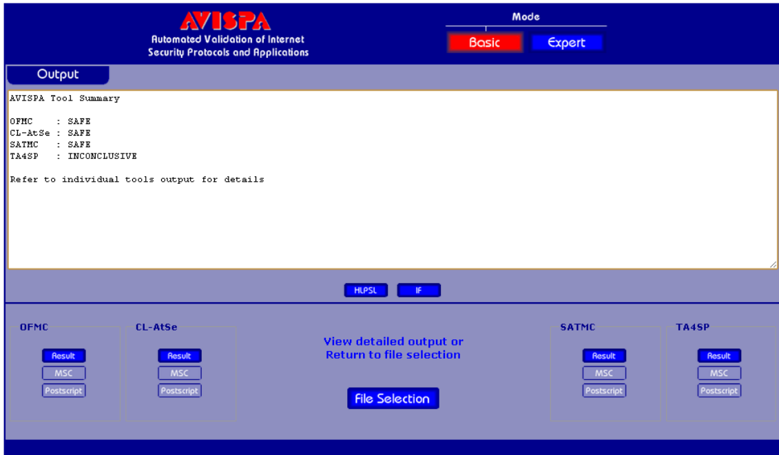
Figure 5.5: Result of verifying the proposed protocol using AVISPA tool.
