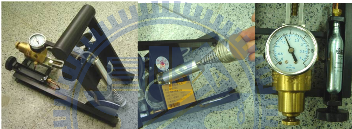
Figure 7 Slipmeter: English XL (left), Neolite testfoot pad (middle), maintain the working pressure at 172kPa (25 psi, right).
