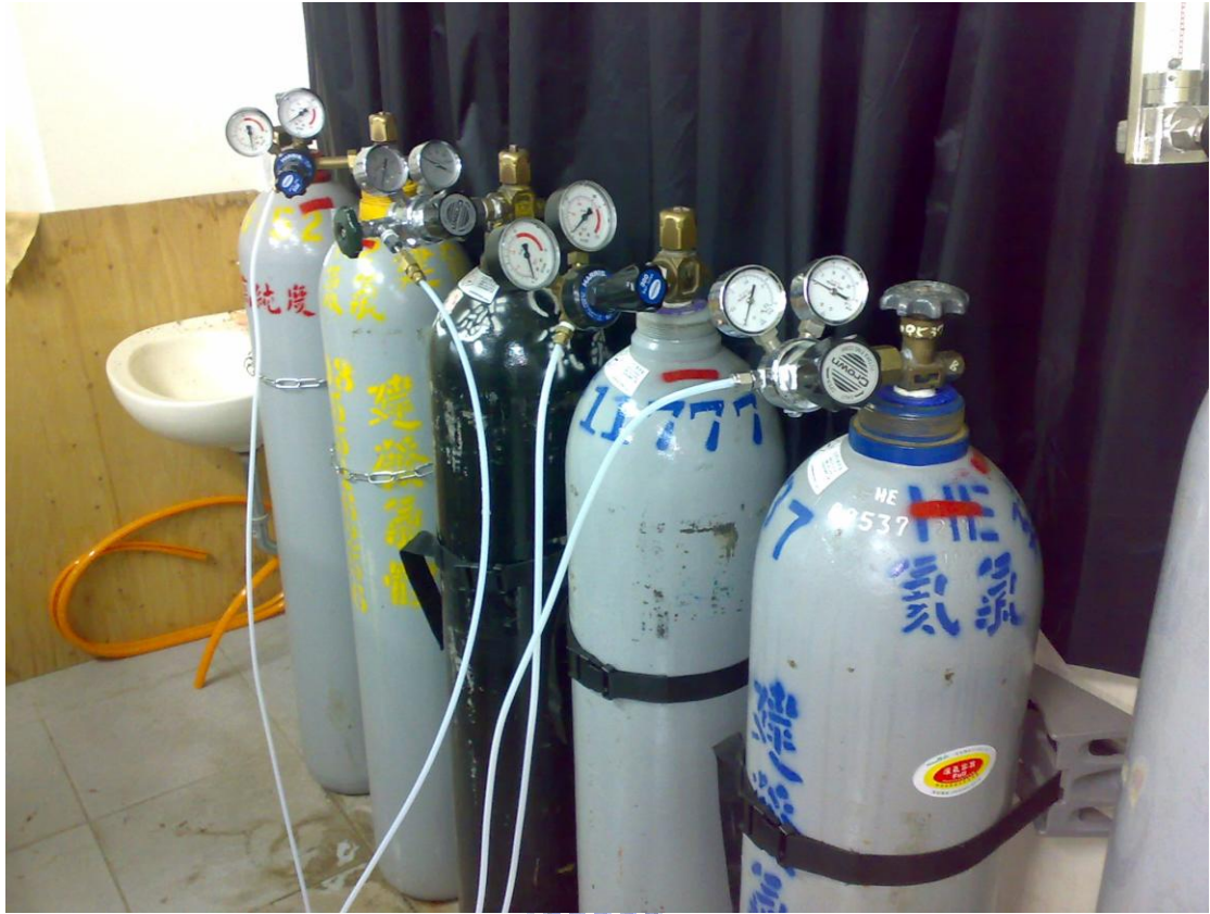
Figure 2.6 Gas feeding system
