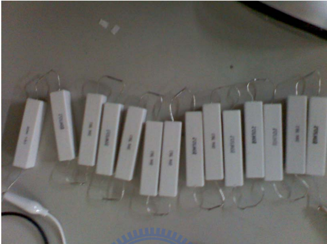
Figure4.3 Cement resistor loads
