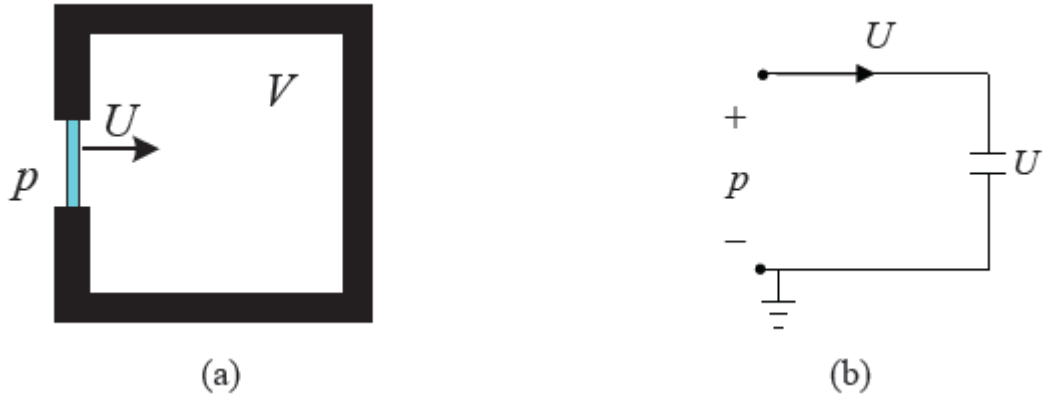
Figure 5. (a) Closed volume of air that acts as acoustic compliance (b) Analogous circuit
