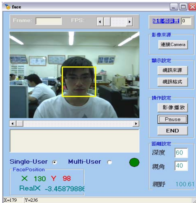
Fig. 21. The GUI of the head tracking system. The system can detect the face and send the coordinate to the beam steering system.
