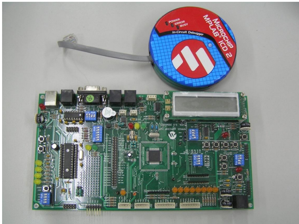
Figure 3- 5: Microchip dsPIC APP021 And ICD2.
