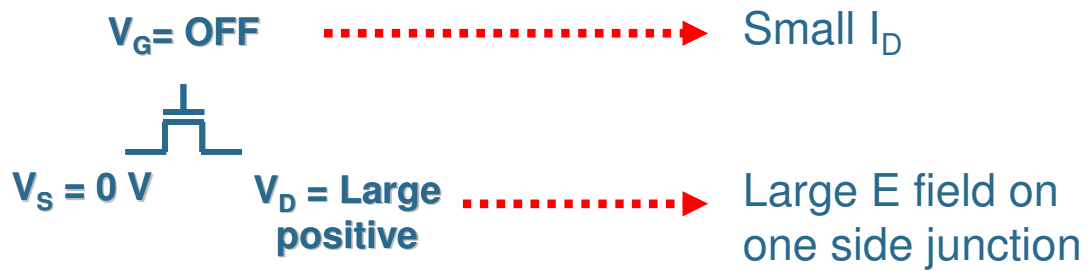
Fig3-20 DC Off region stress for N-Type TFT
