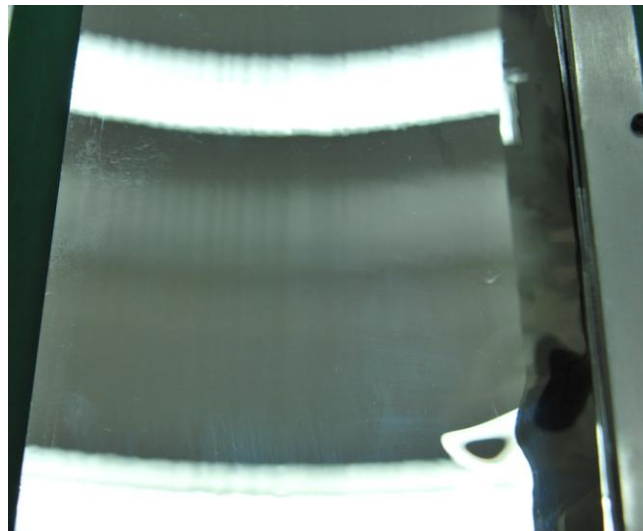
Fig. 5-13 Scratches and notches on the model surface
