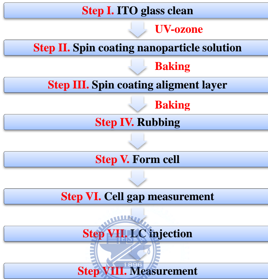
Fig. 4-2 The flowchart of cell fabrication process.
