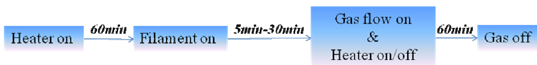
Fig.4.1 The substrate temperature measurement process
