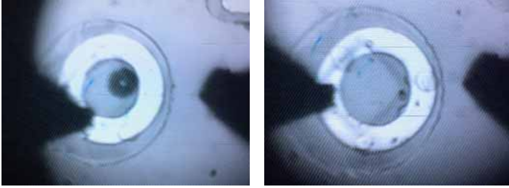
Fig. 3. 19 : The picture of probing contact on PR-filled mesa with and without photonic crystal pattern from CCD monitor.
