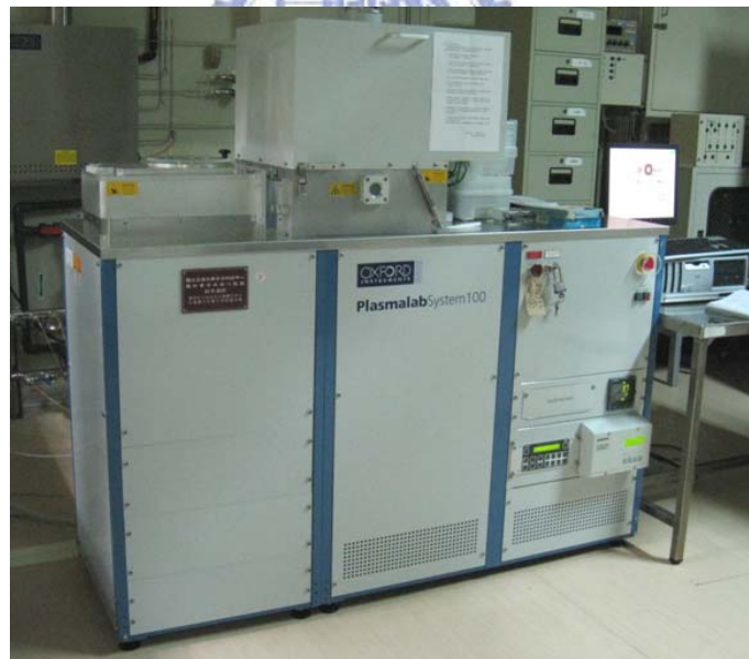
Figure 2-1.3 the high density plasma ICP-RIE system is used for dry etching.
