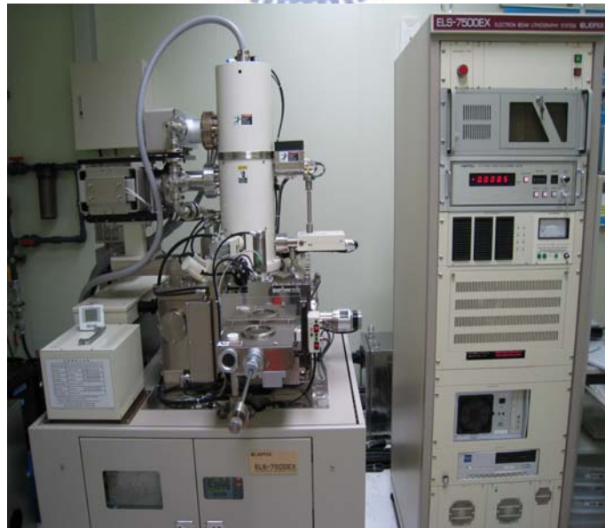
Figure 2-1.1 the nanometer scale photonic crystal patterns is obtained and defined through the E-beam system.
