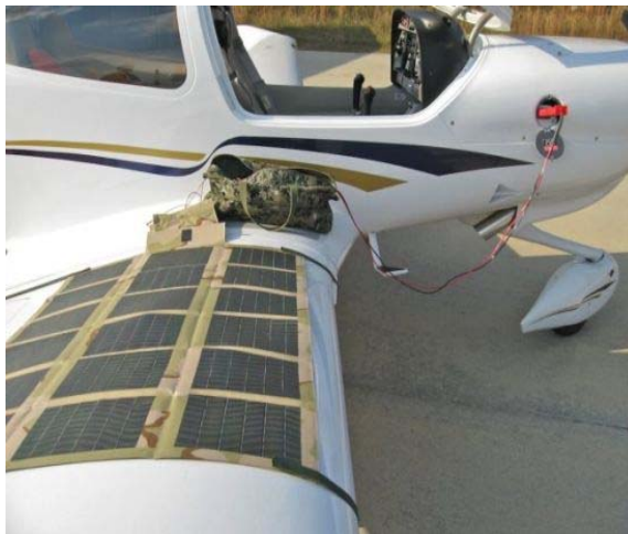
Figure 1-1.2 the flexible sensor or detector array on the airfoil.
