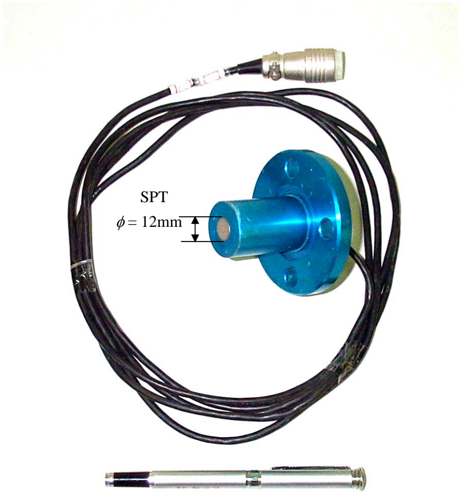
Fig. 3.3. Soil-pressure transducer (Kyowa PGM-02KG) (after Chen, 2003)
