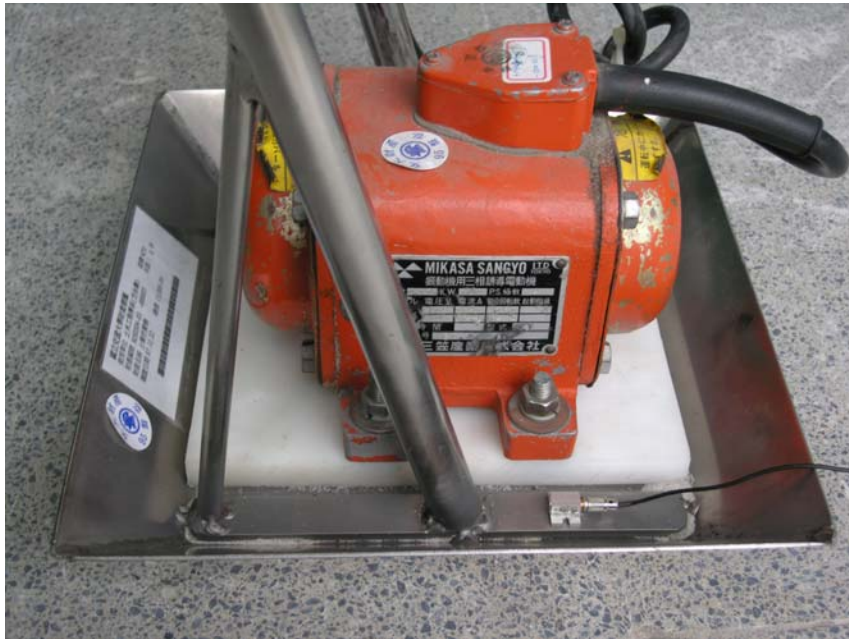
Fig. 5.8. Location of accelerometer to measure a_z
