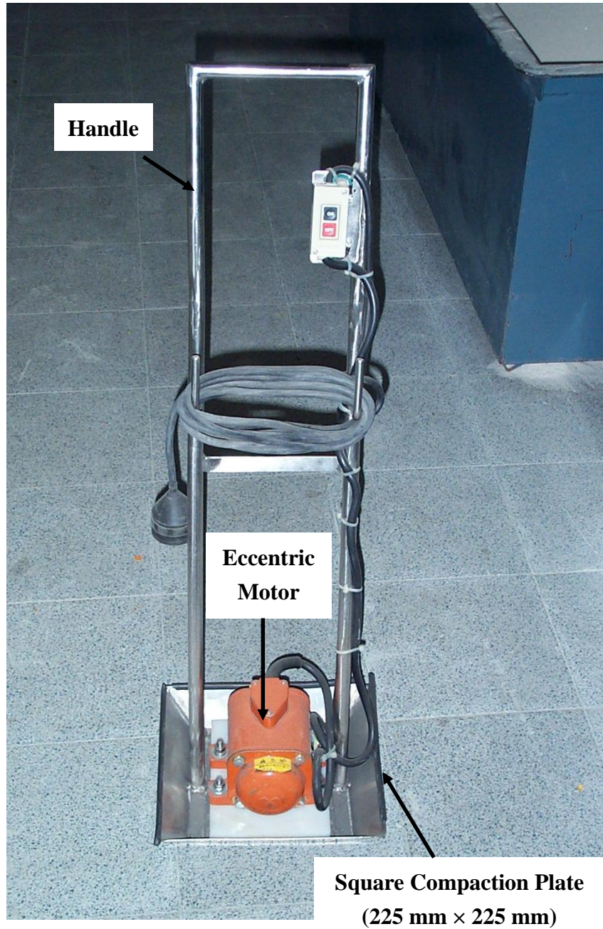
Fig. 3.7. Vibratory Soil Compactor (after Chen, 2002)
