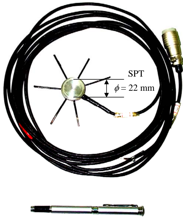
Fig. 3.4. Soil-Pressure Transducer (Kyowa BE-2KCM17) (after Chen, 2003)
