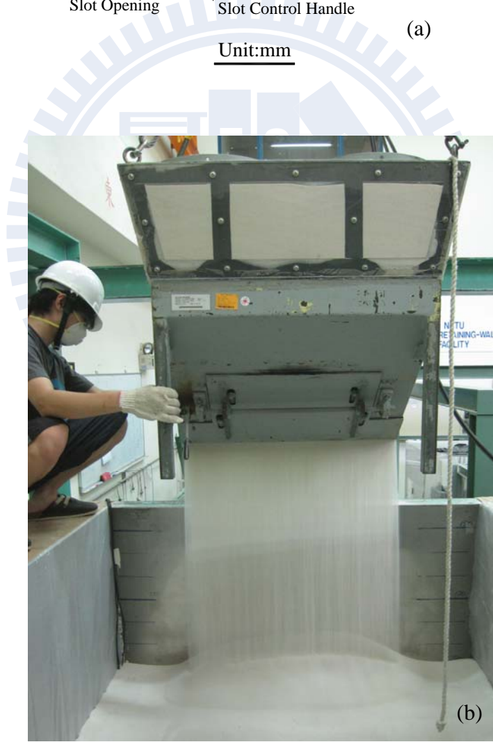
Fig. 4.9. Raining of sand from soil hopper
