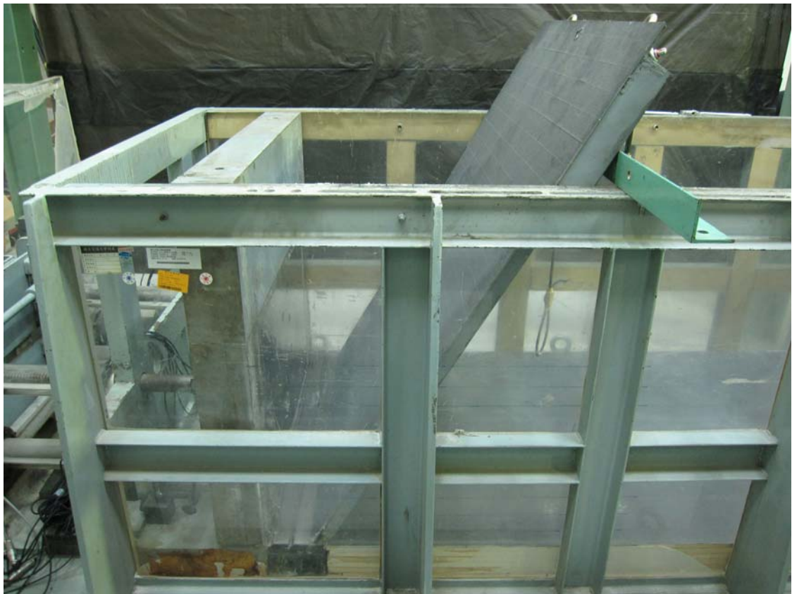
Fig. 6.52. Model wall test with interface inclination \beta = 60^\circ and b = 100 mm
