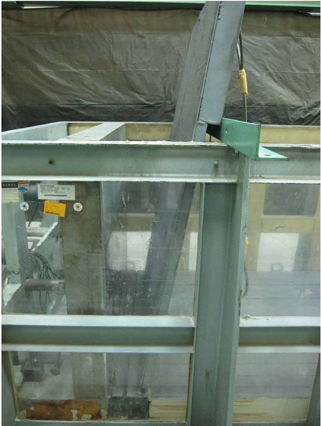
Fig. 6.54. Model wall test with interface inclination \beta = 80^\circ and b = 100 mm
