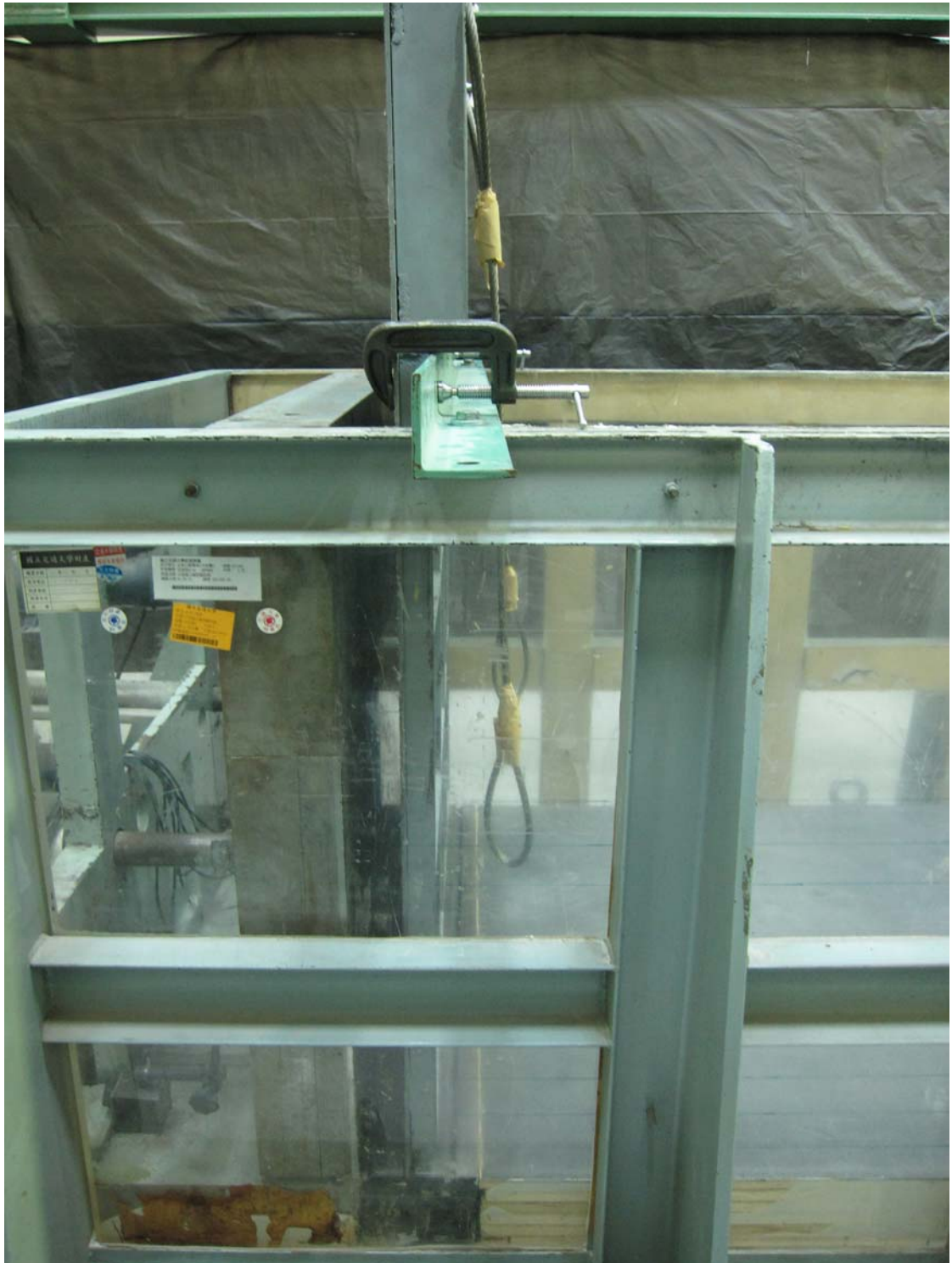
Fig. 6.30. Model wall test with interface inclination \beta = 90^0 and b = 50 mm
