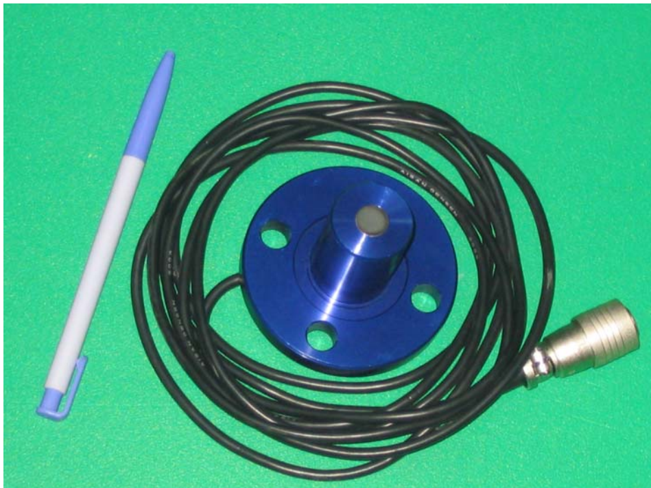
Fig. 3.5. Soil pressure transducer (Kyowa PGM-0.2KG)
