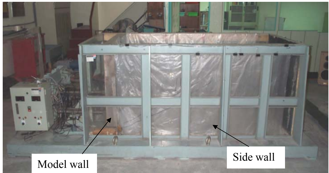
Fig.3.2.Picture of NCTU model retaining wall
