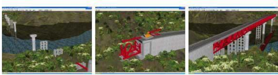
Fig 3.9 A construction stage simulation of truss bridges [Applications of Virtual Reality to Civil and Architectural Engineering Projects, Deyin JIN1, Feng YAN2 and Yuji ITO]
