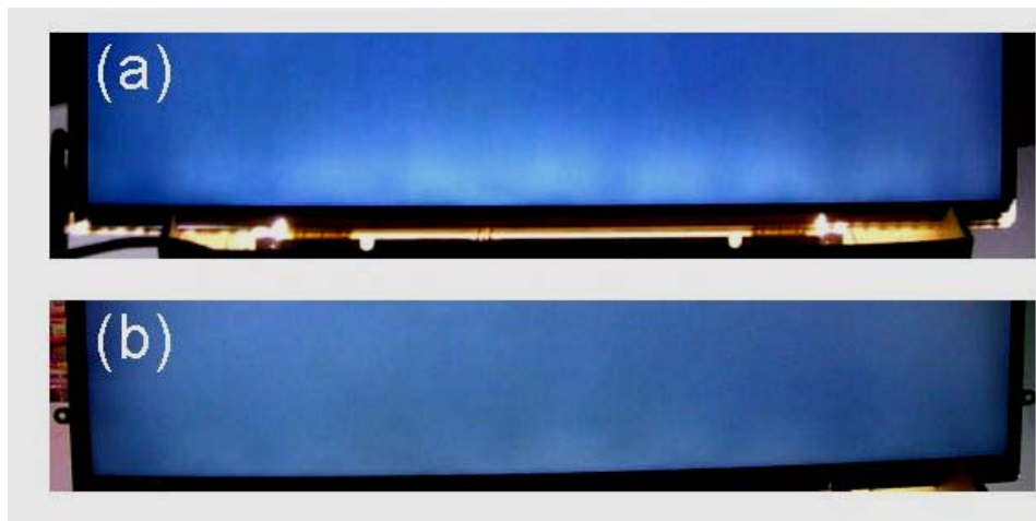
Figure 4.8 Pictures of light leakage phenomenon with ACF bonding temperature at (a) 180°C and (b) 160°C
