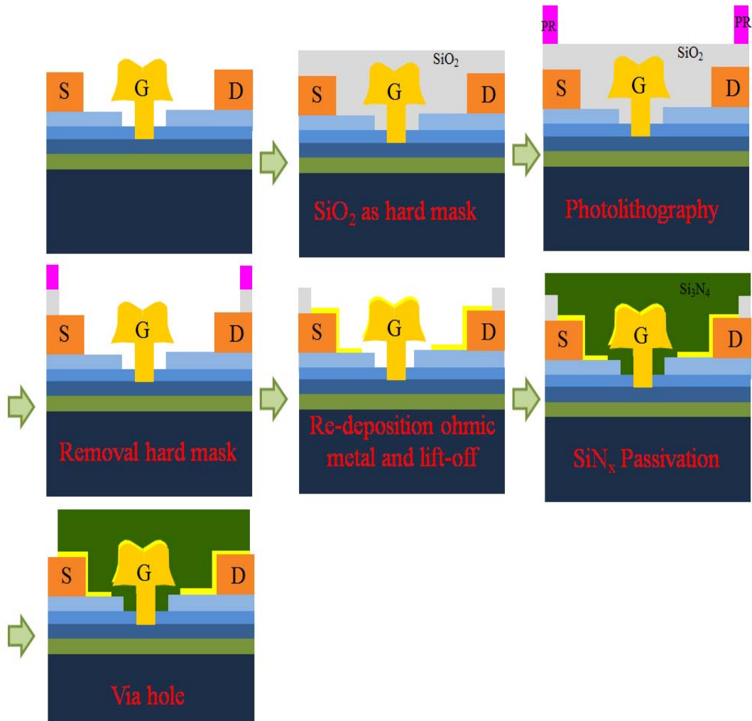
Fig. 2.8 The process flow of self-aligned gate technology for III-V QWFETs
