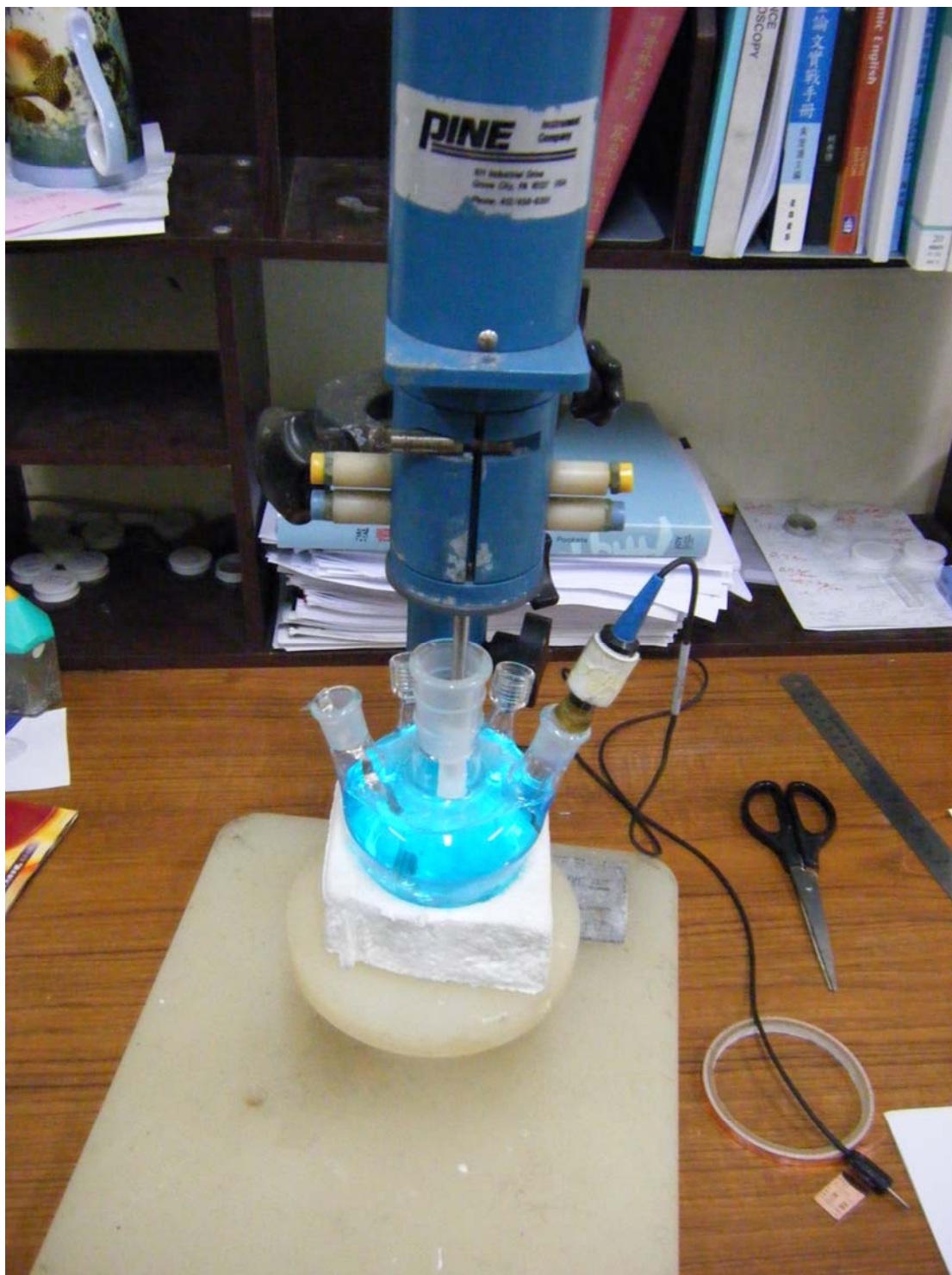
Figure 3-6. A setup for RDE analysis.
