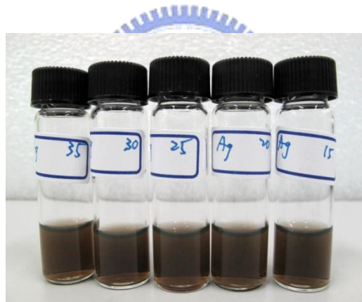
Fig. 4-49 Photographs of aqueous dispersions of Ag nanoparticles after 1 hr reaction time at 60^\circ\text{C} , the samples have less change in color.
