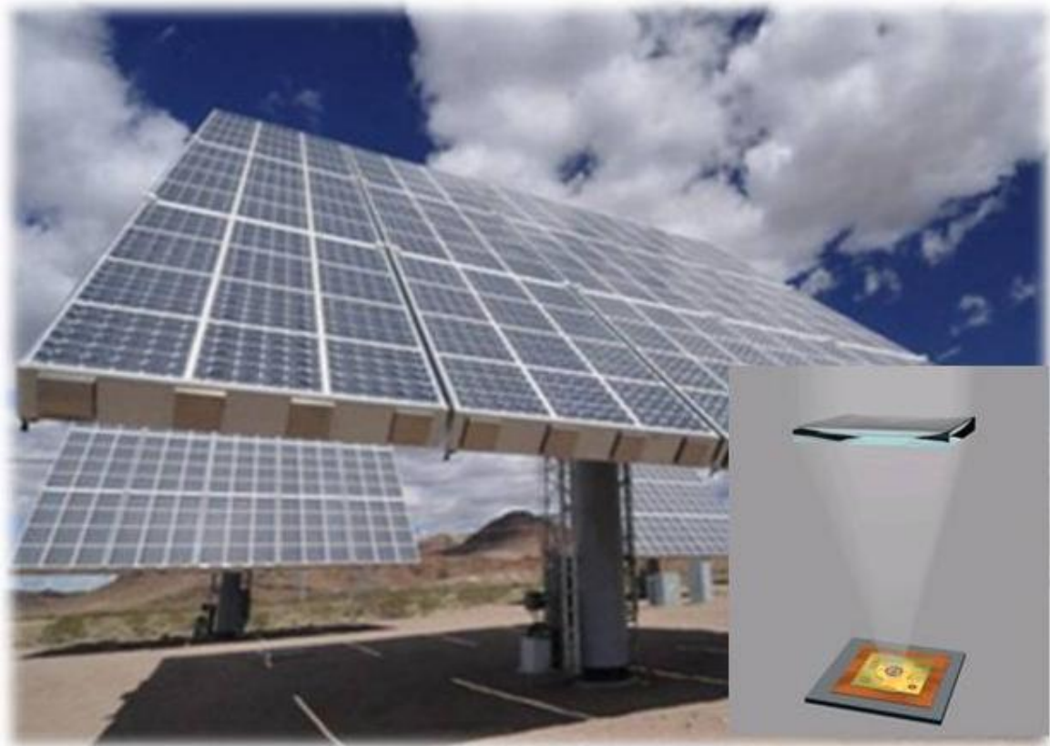
Figure 1-2 Concentrated III-V multijunction solar cells
