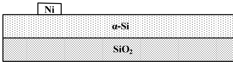
(a) Thermal oxidation, amorphous Si ( \alpha -Si) and Ni deposited
