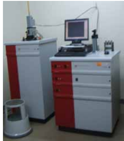
圖 3-1 Quantum Design SQUID Magnetometer MPMS-XL7
