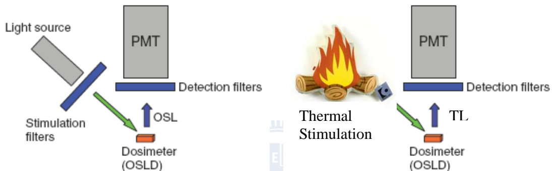
Fig. 1-1. Illustration of operation principle of OSL & TL (a) Optical Stimulated Luminescence (b) Thermal-Luminescence [2].
