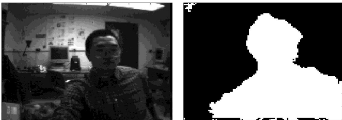
Fig. 2-5 Stereo image based segmentation. Left: original image. Right: processed image [11].
