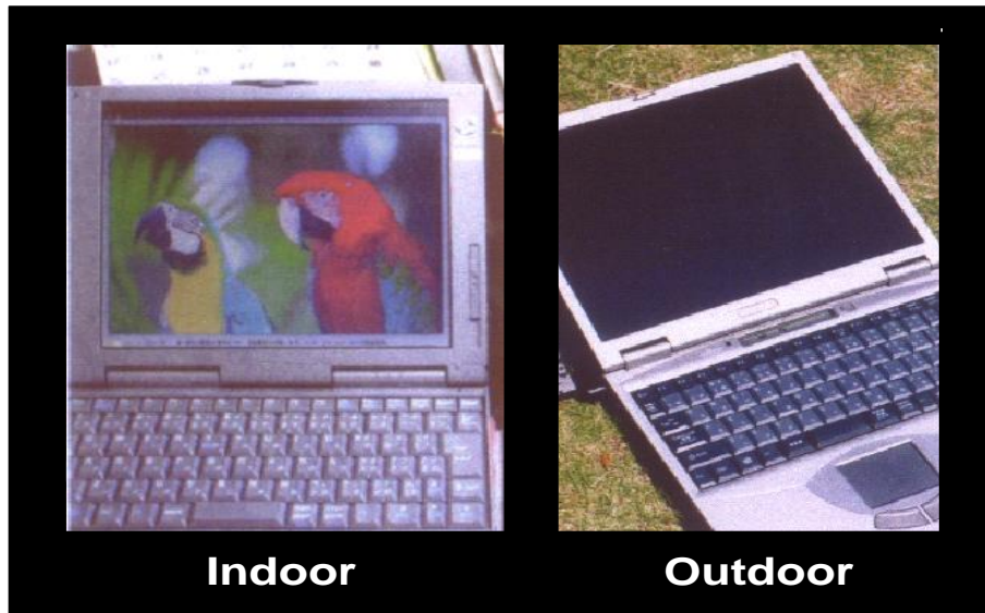
Fig 1-3. The photos of a transmissive type LCD at the indoor and outdoor circumstance
