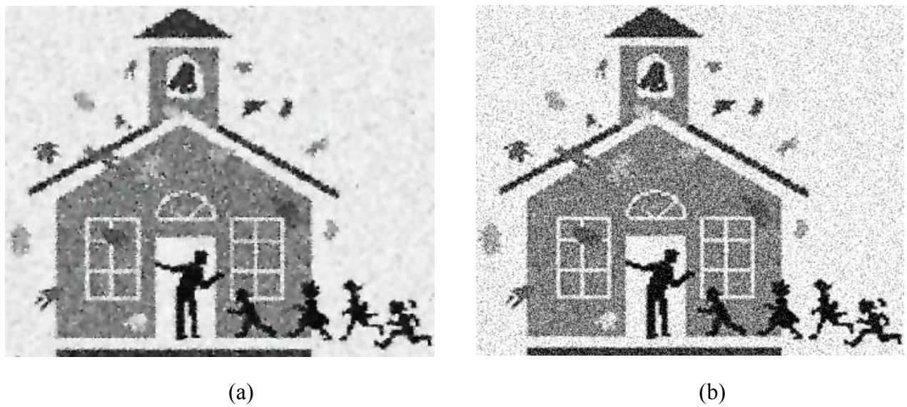
Fig. 5.13 (a) Original image and (b) grayscale image captured by the test chip under the white light intensity of 24 lux and V_{com} of 1.79 V.
