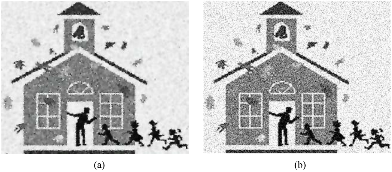
Fig. 4.14 (a) Original image and (b) grayscale image captured by the test chip under the white light intensity of 24 lux and V_{com} of 1.79 V.
