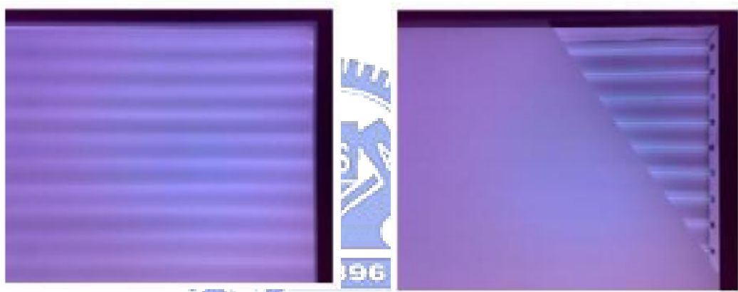
(a) CCFL Slim BL-obvious lamp mura (b) UFL System-Invisible Lamp mura
