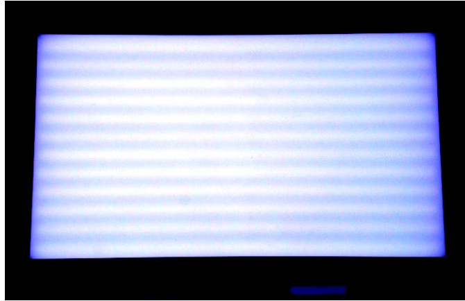
Fig. 1-3 Lamp-Mura defect of a 32-inch direct-emitting CCFL backlight systems captured by a charge-coupled device (CCD).
