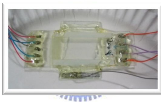
Fig. 5-1 The multi-electrode driven cylindrical LC lens sample (MeDLC)
