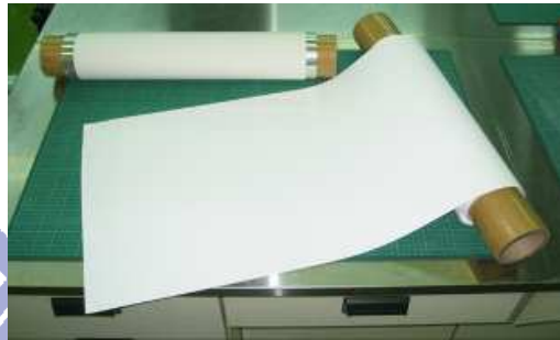
Fig. 3-4 (a) The remote phosphor converter (RPC); (b) the coated PET films with trichromatic phosphor.
