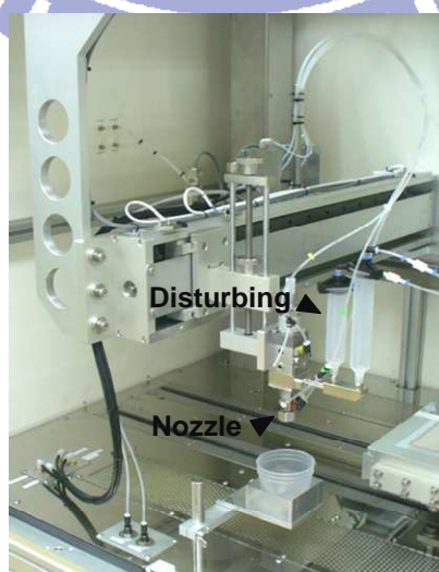
Fig. 3-7 Mechanical structure of pulsed-spray coater.
