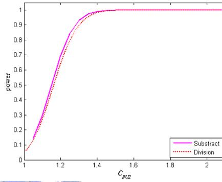
Fig 6. Power curves of the two methods for  $C_{PU1} = 1.00$  and  $n_1 = n_2 = 150$ .
