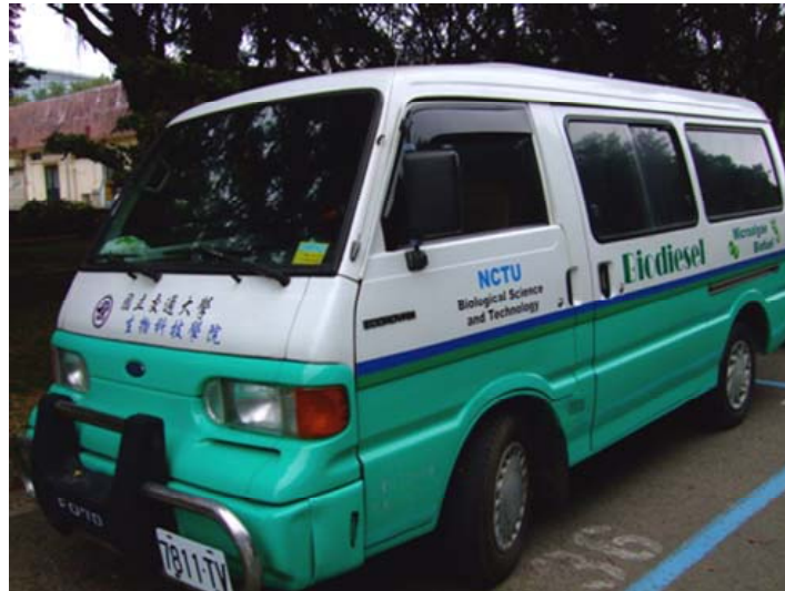
Figure 3-18. Figure of microalgal oil and biodiesel car. A, shows the microalgal oil form N. oculata . B, shows the biodiesel car of our laboratory. The highest diesel/biodiesel mixed ratio added in the car was B70 and the mileage by biodiesel is over 1,000 kilometers.
