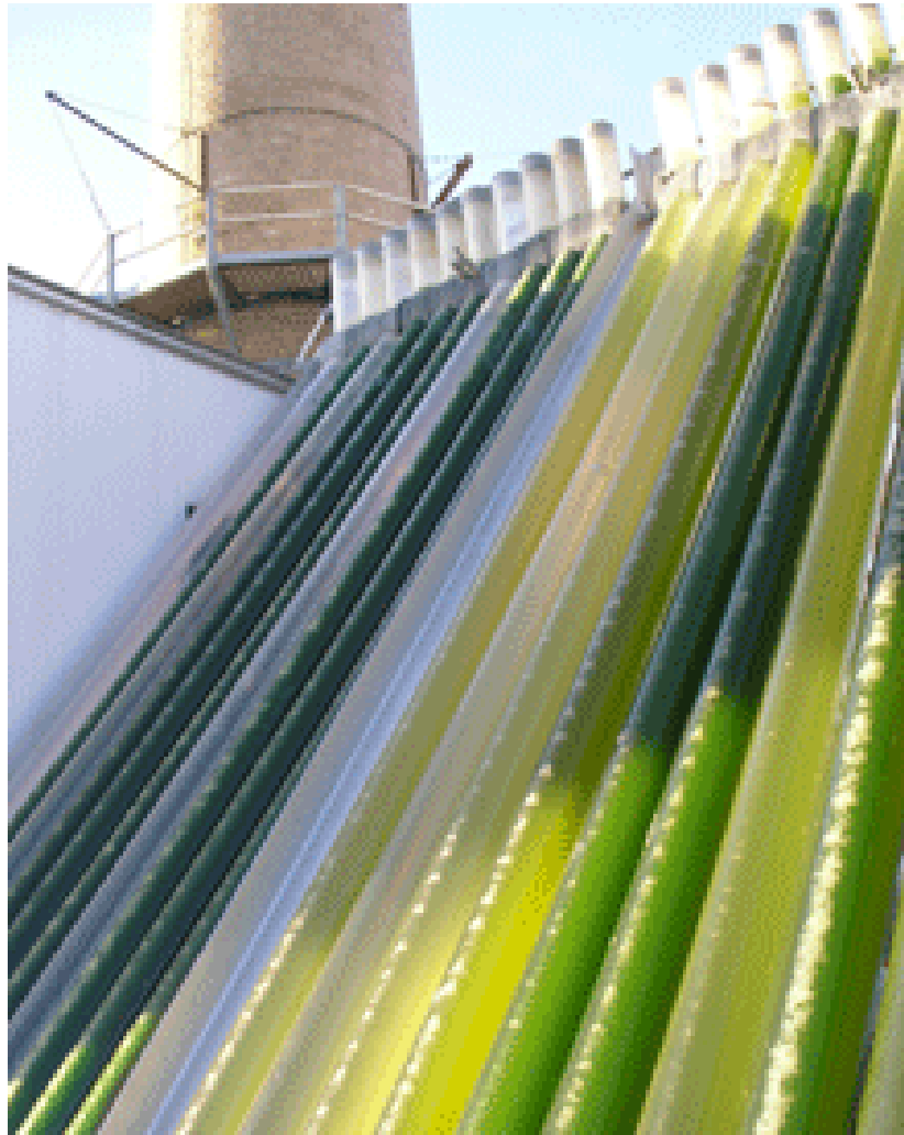
Figure 1-3. Closed column type photobioreactor fed with recycled CO 2 from smokestack, fermentation, and geothermal gases production plant in MA, USA.
