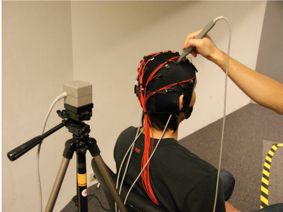
Figure 7. Channel location recording by 3D digitizer system. A photograph shows the 3D digitizer system for digitizing and recording the real locations of each channel in individual subject. The processing is described as following. While we measured the 3D position of the channels, we mounted the transmitter behind the subject and put the 3 receivers under the Oz, T3, and T4 channel inside the electrode cap. The transmitter should far from the metallic surface and located in close proximity to the receivers. Beside, we routed the transmitter cable separate from the receiver cables in order to avoid possible noise problems. After these setups, we used the stylus to point out each channels and recorded the 3D channel locations.
