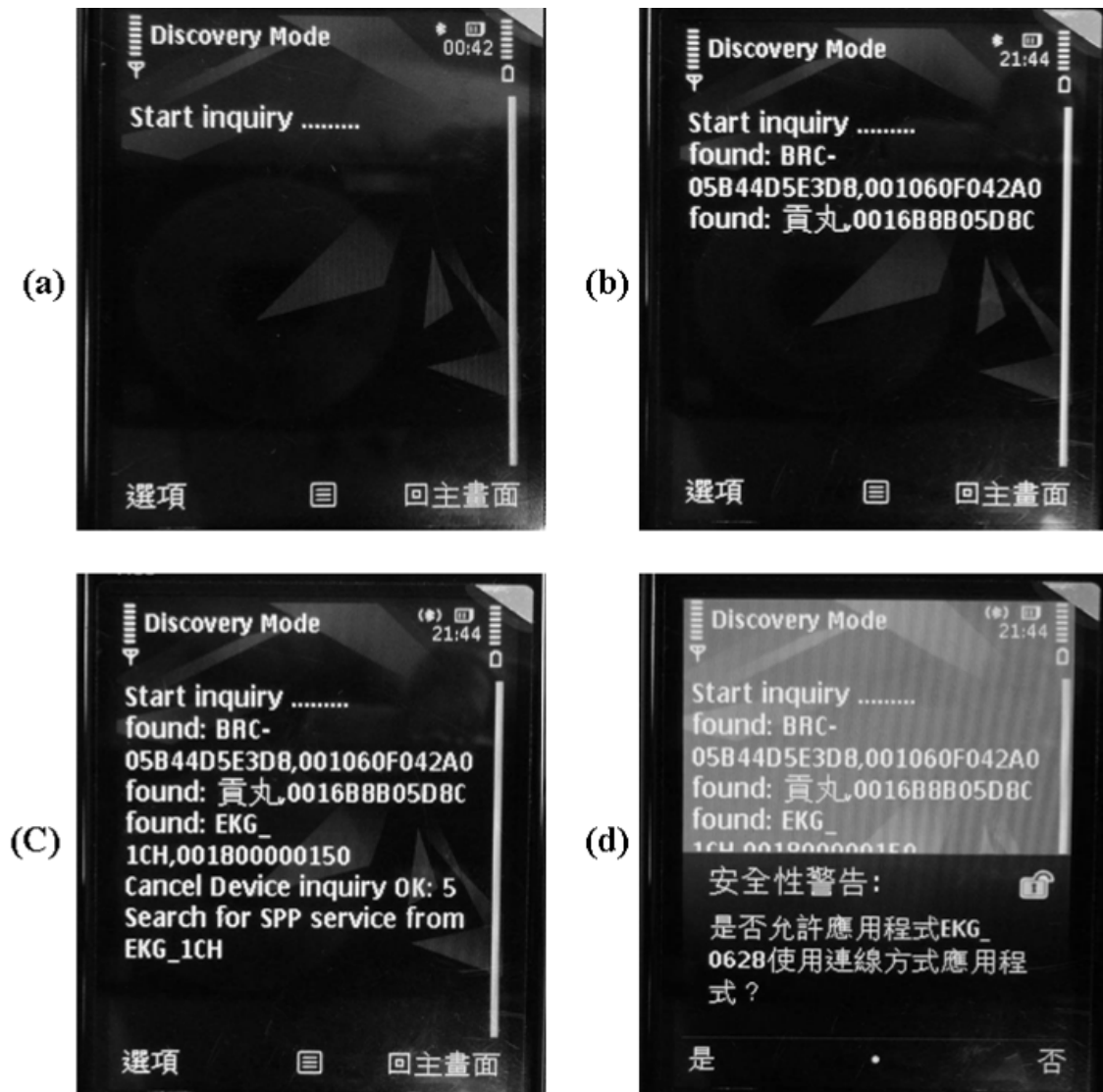
Fig.3- 18 Snapshot of searching ECG acquisition module process: (a) start to inquiry the Bluetooth device around, (b) lists the device found around, (c) found the ECG acquisition module, and try to search the SPP service, and (d) found SPP service and try to create the connection.
