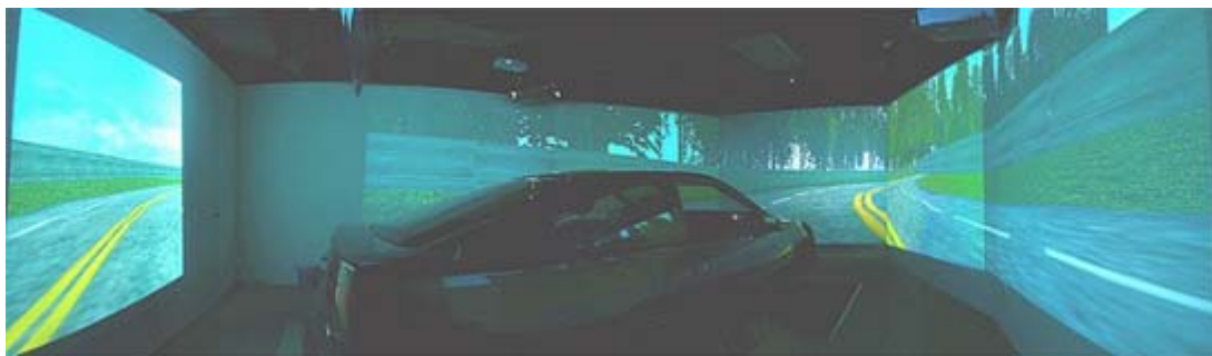
Fig. 2-4: The picture showed the overview of surrounded VR scene. The VR-based four-lane highway scenes were projected into surround screen by seven projectors.
