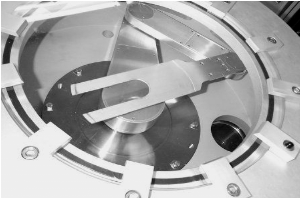
Fig. 2-4 Photograph showing the robot arm in the transfer chamber.
