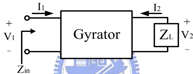
Fig. 2.13 The two port network of Gyrator
