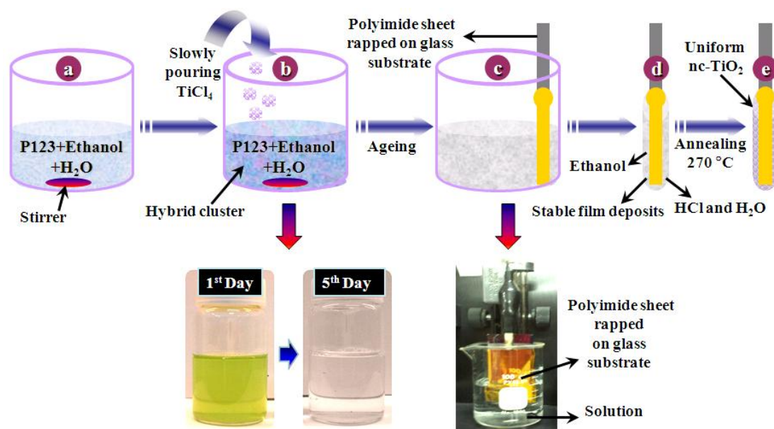
Figure 6.1 (a-e) Schematic illustration of the proposed synthetic solution proceeded dip-coating approach for the preparation of the uniformed nc-TiO 2 film presented in this work.
