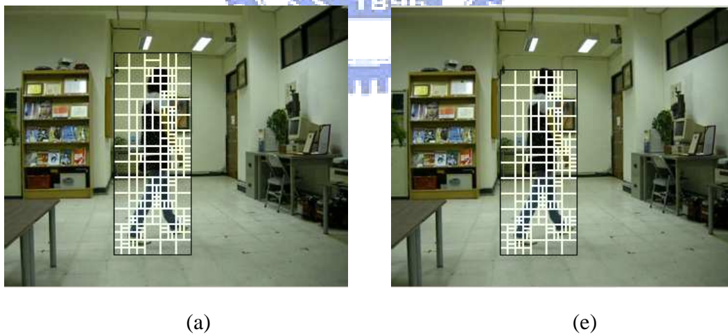
Figure 3.4 An example of the results of applying the range reduction algorithm. The black rectangle is the motion region and the white rectangles are the sub-macroblocks in the region. (a) The first P frame without reduction. (b) The second P frame without reduction. (c) The third P frame without reduction. (d) The 4th P frame without reduction. (e) The first P frame with reduction. (f) The second P frame with reduction. (g) The third P frame with reduction. (h) The 4th P frame without reduction.
