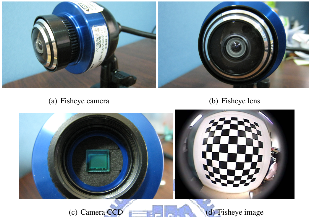
Figure 2.2: Fisheye camera, 1.7mm focal length lens, 1/2 inch CCD and image shoot by fisheye camera. (a) This is the fisheye camera we use. (b)(c) The focal length of the fisheye lens is 1.7mm, and inside the camera is a 1/2 inch CCD. This combination allow our camera to capture a 180 degree viewing angle. (d) This image is captured by our fisheye camera. The chess board calibration pattern is distorted due to the refraction of the fisheye lens.
