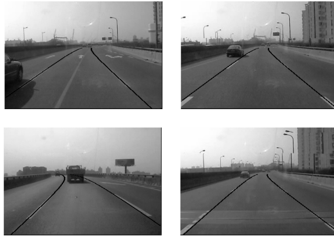
Figure 1.1: Examples of lane detection. On the freeway, the lanes are detected to determine the lateral position of the vehicle.
