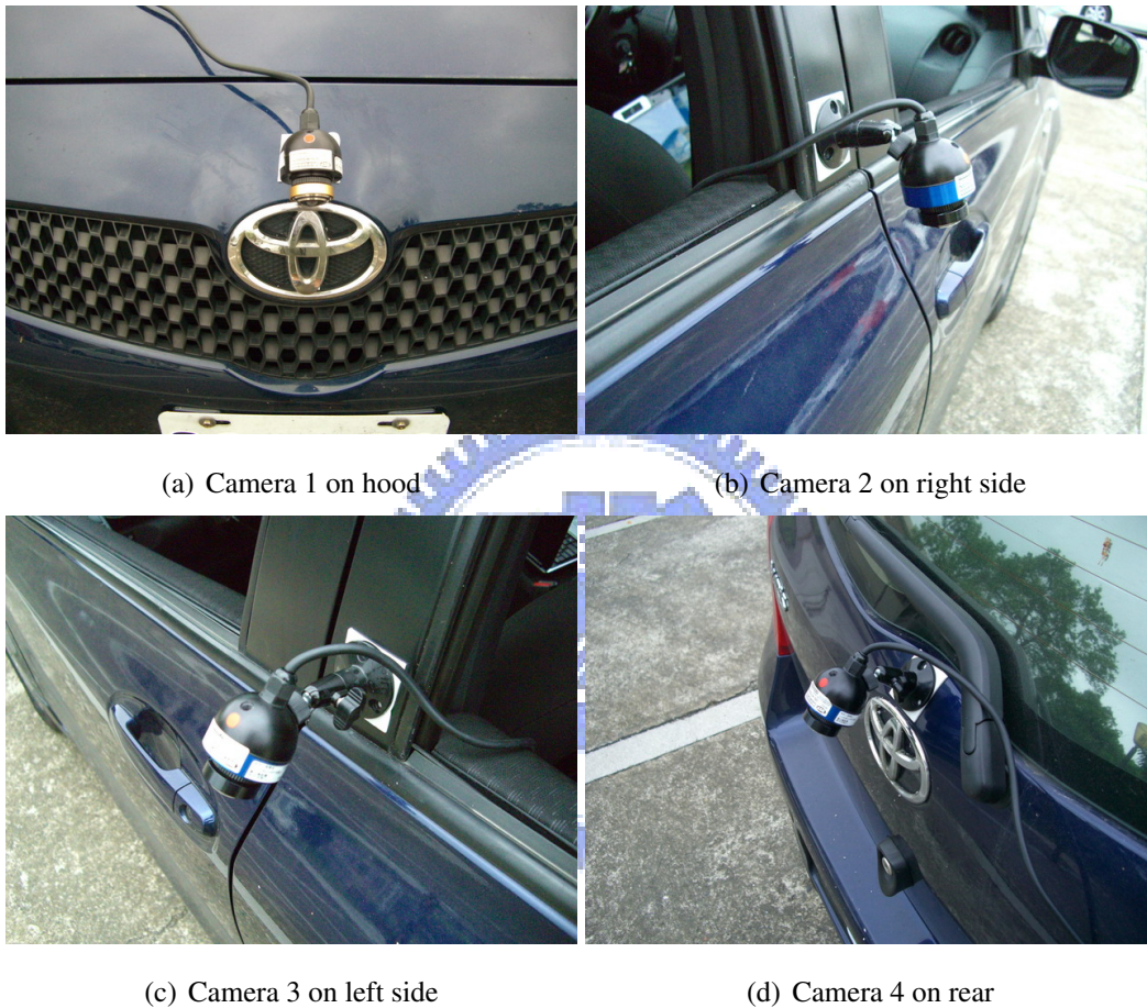
Figure 2.5: Four fisheye cameras are mounted on the middle of each side to obtain the surrounding scenes. (a) Camera 1 for front view. (b) Camera 2 for the view of right side. (c) Camera 3 for the view of left side. (d) Camera 4 for rear view.
