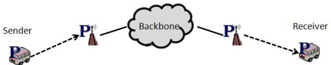
圖 3.20 An SMFS scenario where the Sender node can Directly Communicate with RSU node
