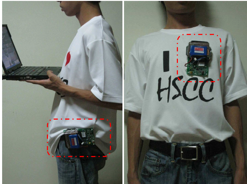
Figure 2.1: mounting sensor device on waist or hanging on chest.
