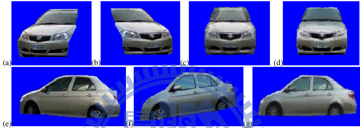
Fig. 24 (a) Segmented image of front region, (b) mirror image of (a), (c) synthesized car image from (a) and (b) by mirror morphing, (d) synthesized template car image, (e) segmented image of side region, (f) selected mirror template, (g) synthesized car image from (e) and (f) by quasi mirror morphing
