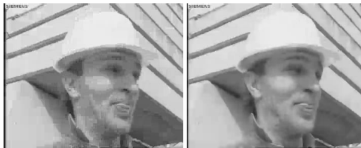
Fig. 2.12 Performance of the deblocking filter for highly compressed pictures [2] Left: without deblocking filter, right: with deblocking filter
