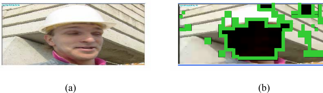
Fig. 4.13 Regions in the top field that are referred by MB’s in the bottom field
