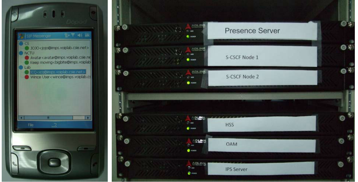
Figure 1.2: Instant Messaging and Presence Service System
