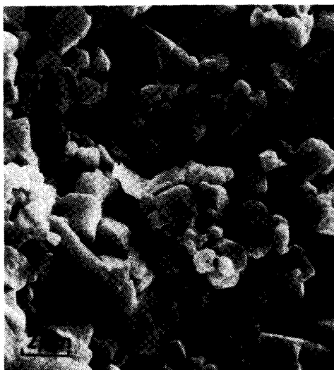
Fig. 1. Scanning electron micrograph of fracture surface of the BSK sintered compact.
