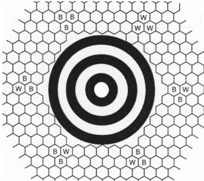
Fig. 2.6 The orientation patterns relative to the finder pattern, the orientation patterns are marked by W and B.
