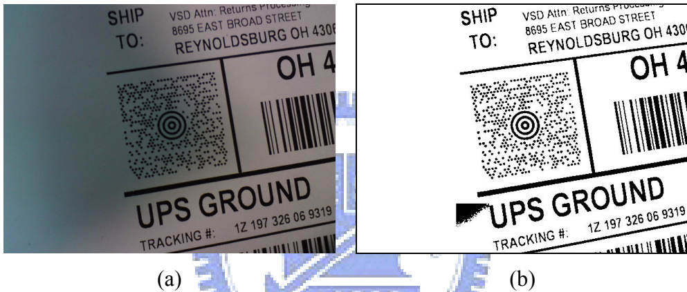
Fig. 2.14 An example of minimum mean square error thresholding. (a) A MaxiCode image. (b) The binary image of (a).
